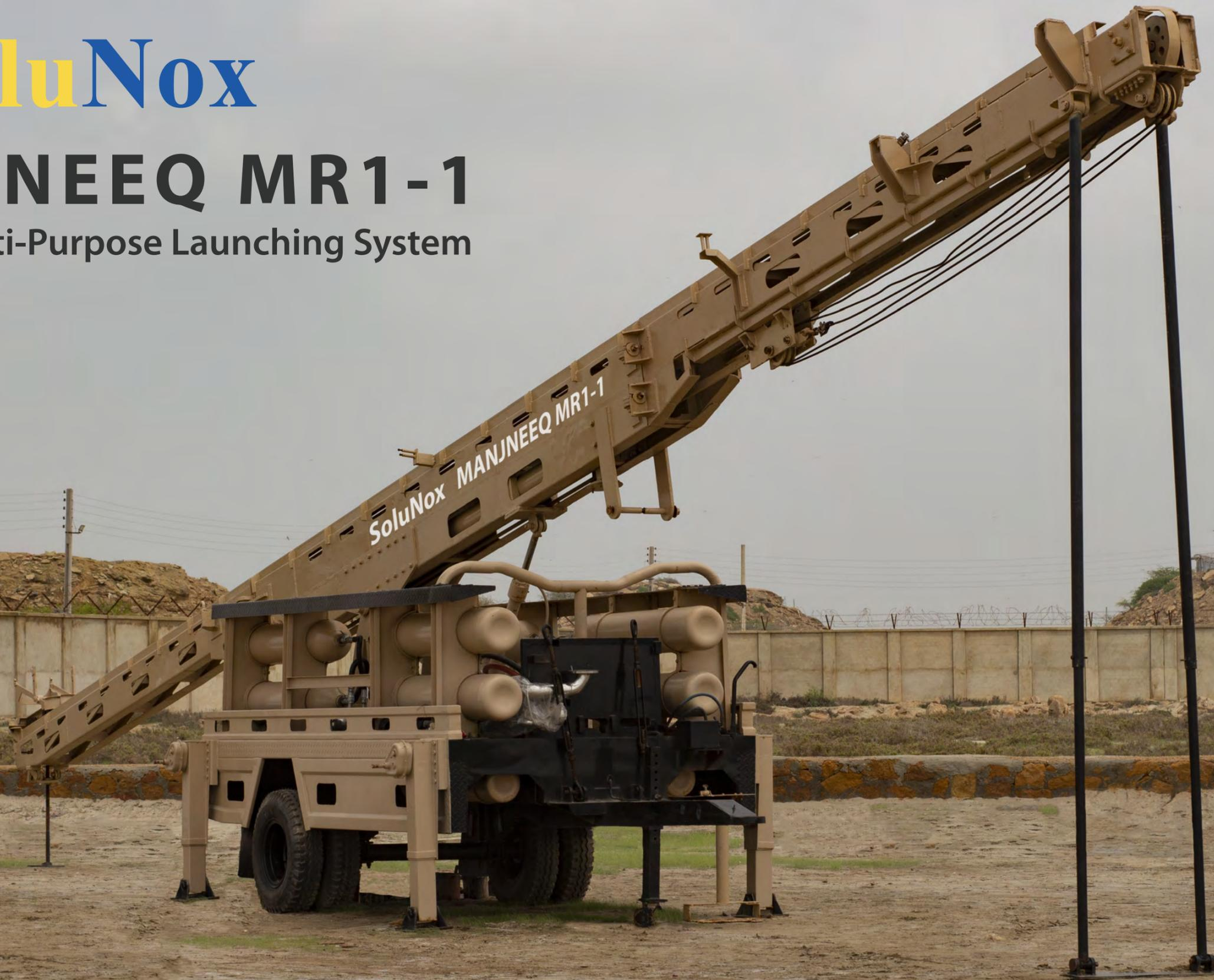
When performance and efficiency cannot be compromised 'MANJNEEQ MR1-1' is the ultimate solution, developed in joint collaboration with SoluNox launching Systems and Pakistan Aeronautical Complex Kamra. It is designed to meet the current and emerging operational requirements of optimized launch for up to Group-III (less than 1350kg and less than 250 kts) Unmanned Aerial Systems and Target Drones
