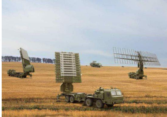
Fig. X.10 The Nebo-M radar complex, comprising 3 radars in different bands (metric, deca-metric and centimetric, in terms of wavelength, or VHF, L and S/X, in terms of frequency) and a control station, performing sensor fusion [19, 23]
