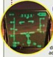
**6 WIDE-ANGLE HUD:** A pilot can either look out the cockpit window or put his head down to scan flight instruments. Head-Up Display lets him do both together by displaying flight data across windshield
