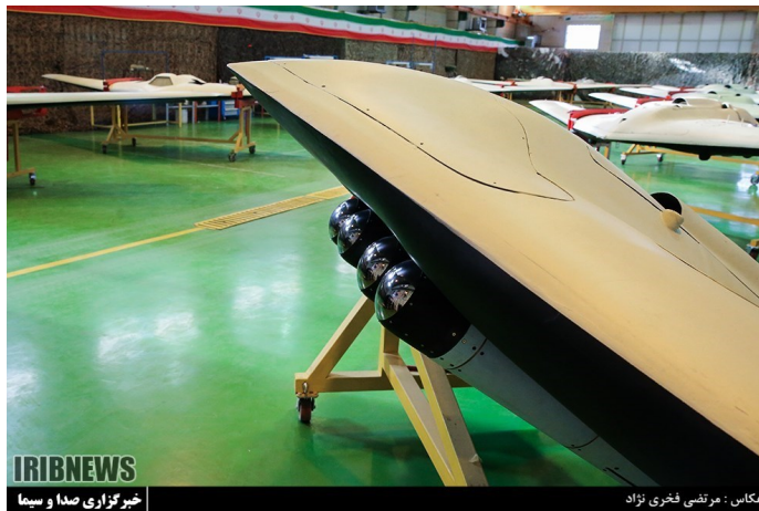
An example of an Iranian RQ-170 flying drone equipped with four smart point bombs under the fuselage
