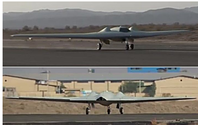
s UAV tests with a wheeled and retractable landing gear in the fuselage'171
