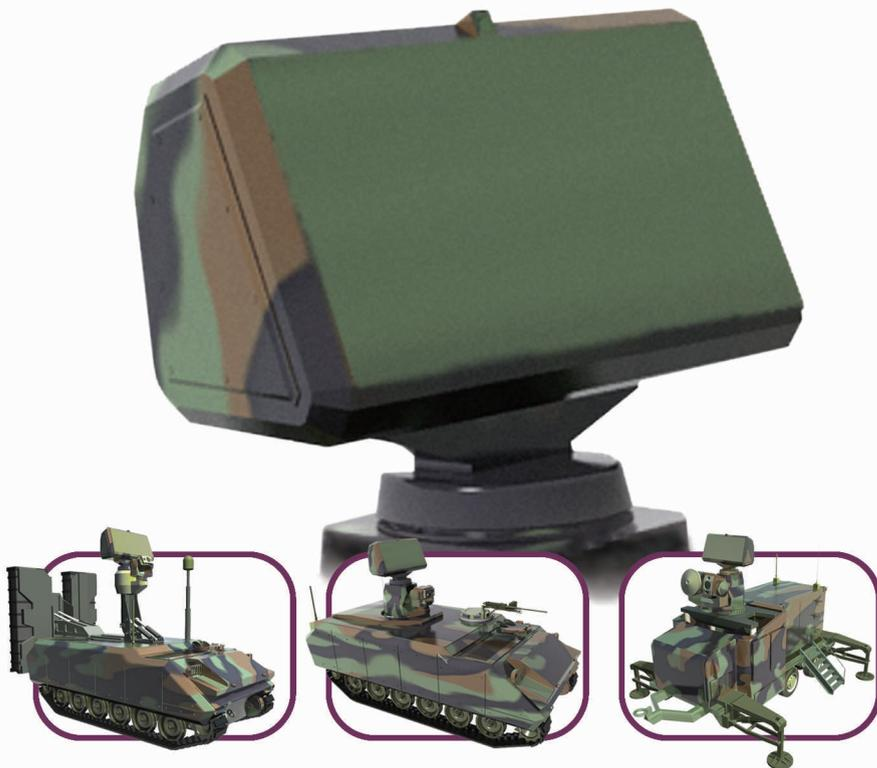
ASELAN Mobile Search Radar is ASELAN's latest 3D radar designed for mobile air defense weapon systems with modern radar design technologies such as digital beamforming and solid state transmit/receive modules.
