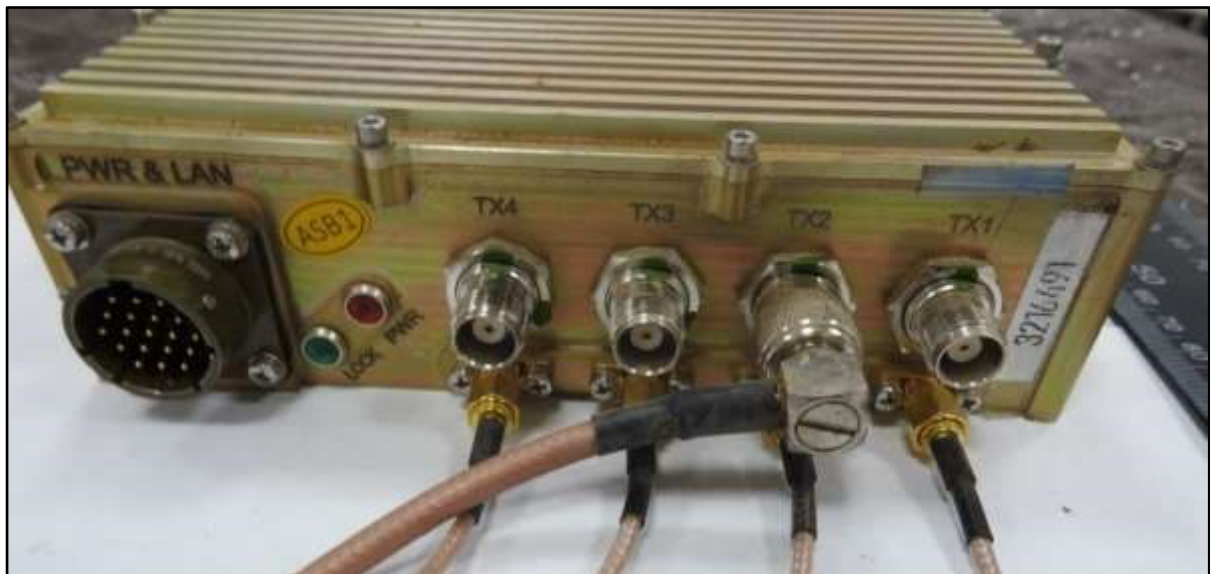
Figure 21. IRN-05 GNSS Transceiver.
