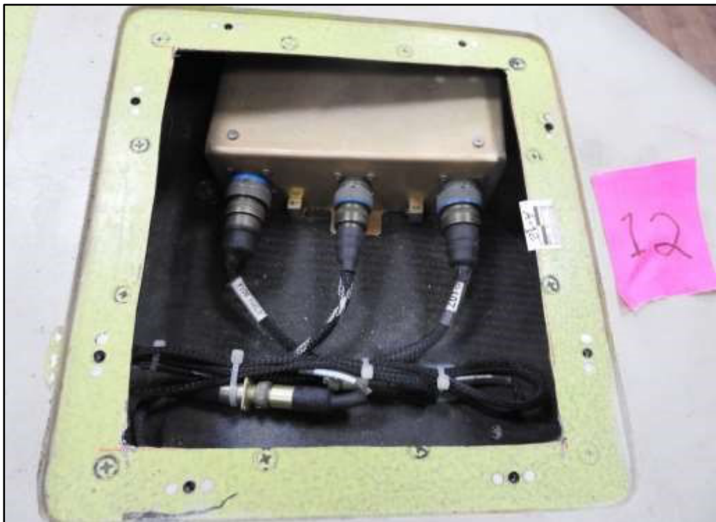
Figure 31. Panel 12 containing Engine Control Unit (ECU).
