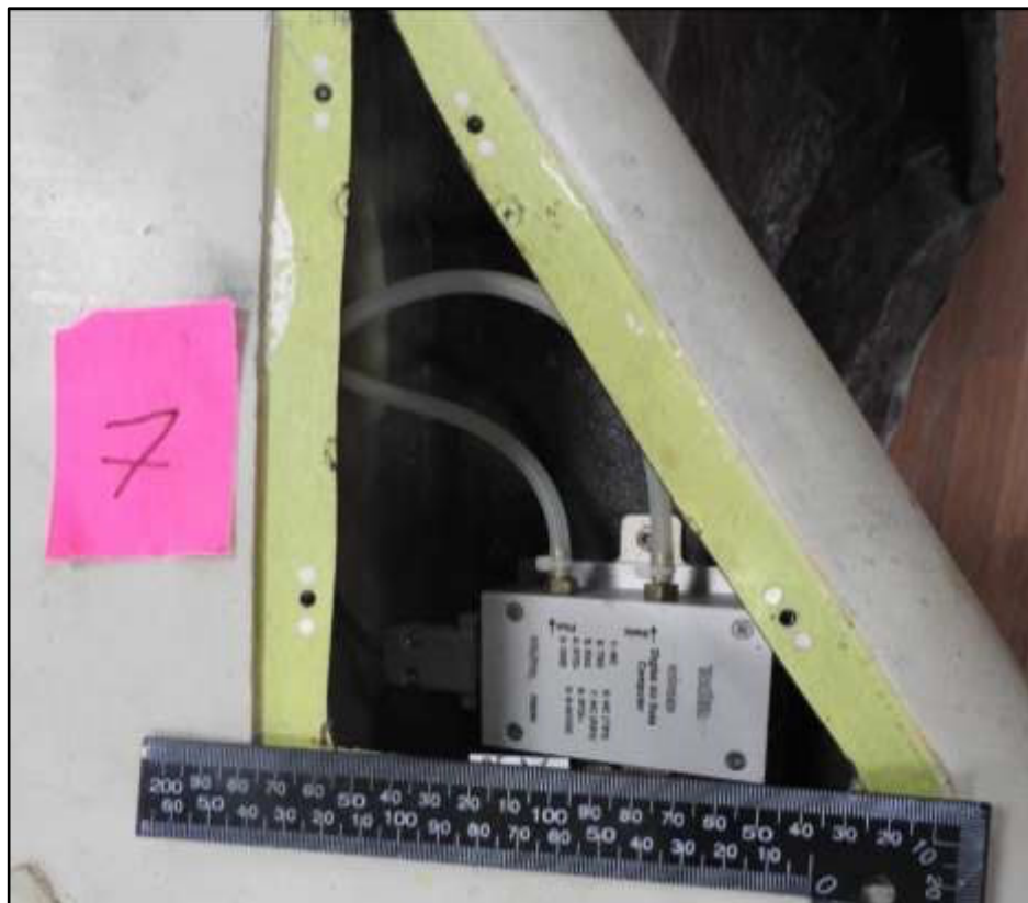
Figure 23. Panel 7 containing Inertia Measurement Unit (IMU).
