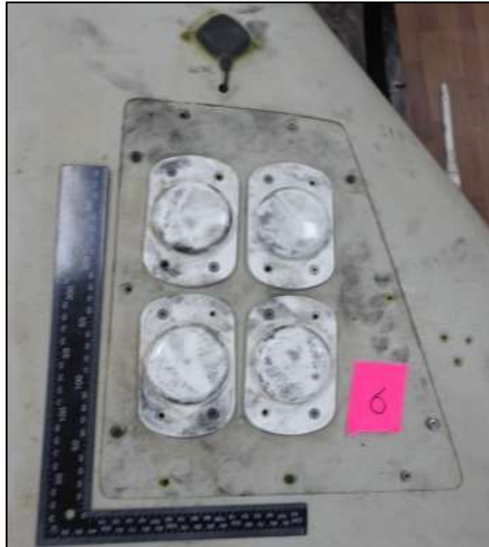
Figure 18. Panel 6 showing four new “hardened” GNSS pucks in white. Figure 18 also shows the old black GNSS puck, which has been cut from the system.
