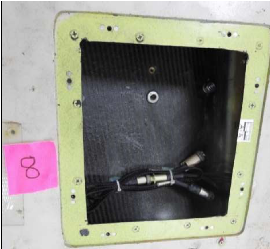
Figure 24. Panel 8 containing connectors for aileron servos.
