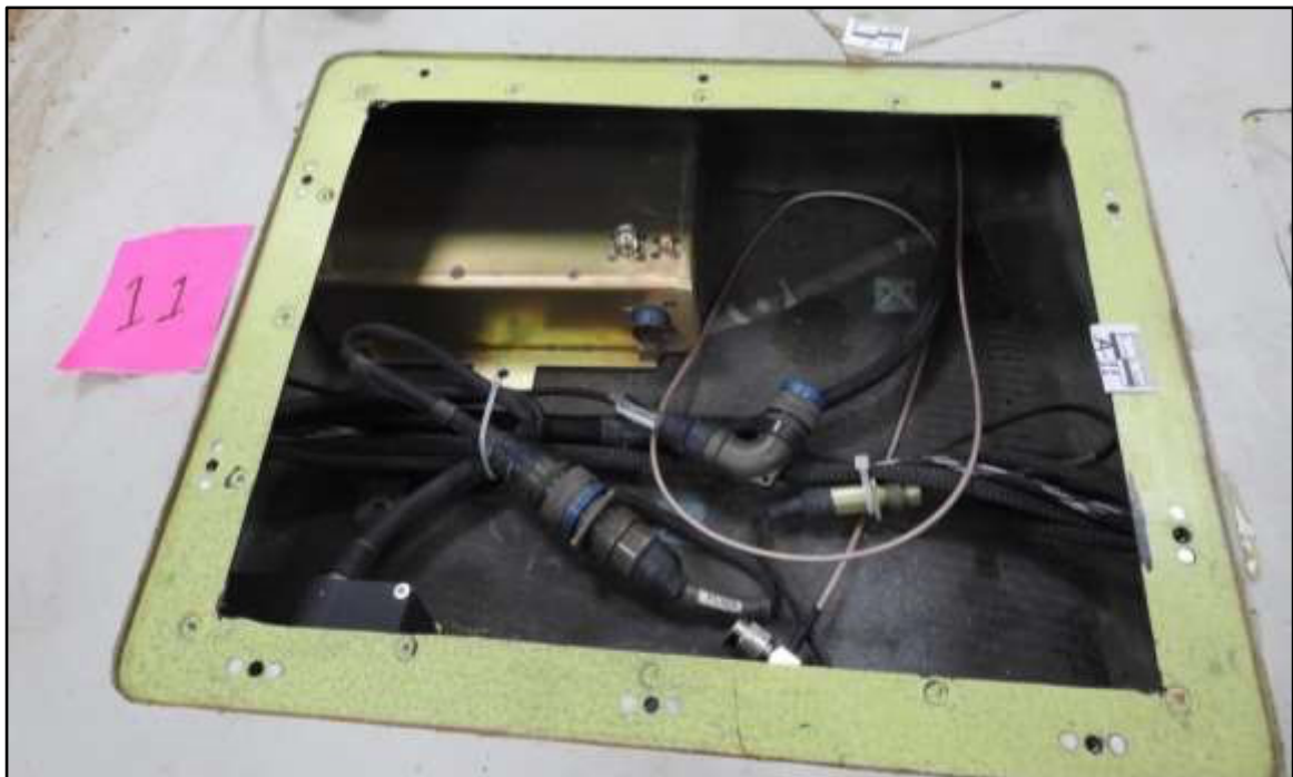
Figure 27. Panel 11 containing ATOL – “Automatic Take Off and Landing”.
