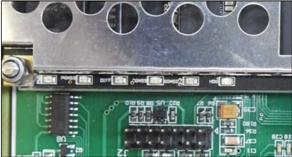
Figure 30. LEDs on ATOL PCB showing “PGNSS, DGNSS, SGNSS, HDG”.
