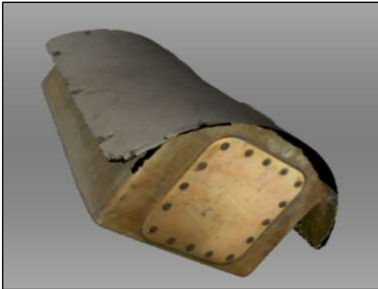
Figure 41. 3D Scan of IRN-05 panel 10 fuel/lubricants tank.
