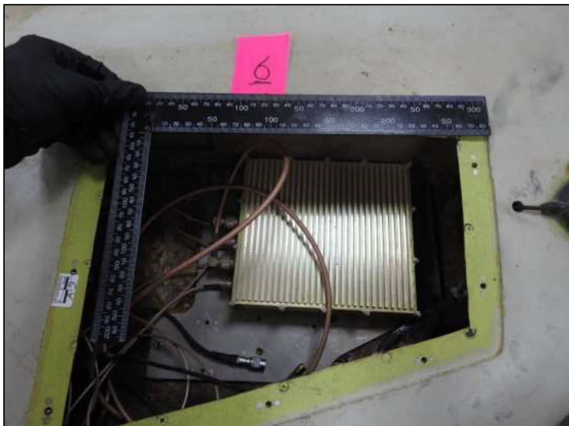
Figure 19. Panel 6, Containing GNSS Transceiver.
