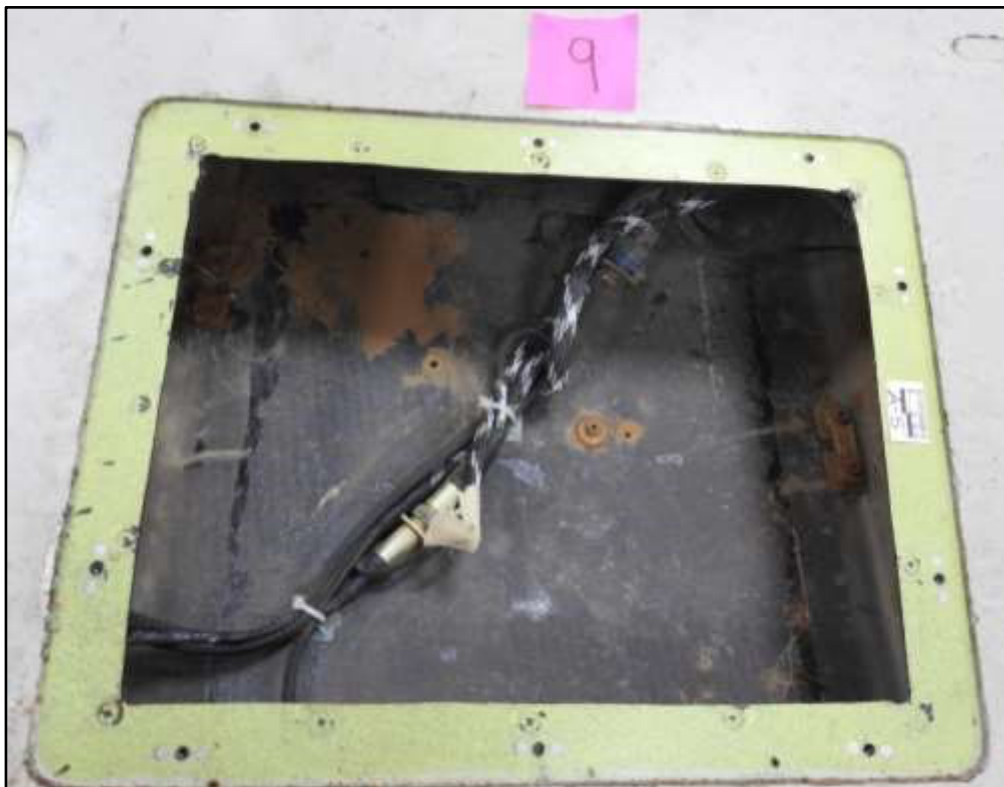
Figure 25. Panel 9 containing wiring loom connectors.
