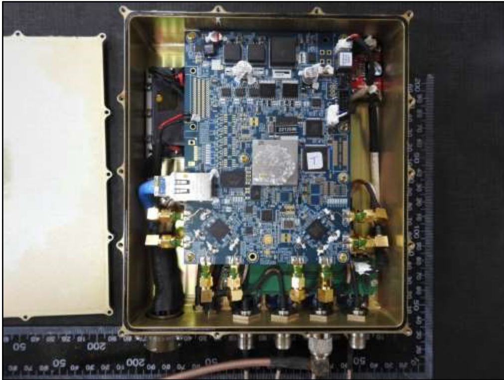
Figure 22. Internal GNSS Transceiver.
