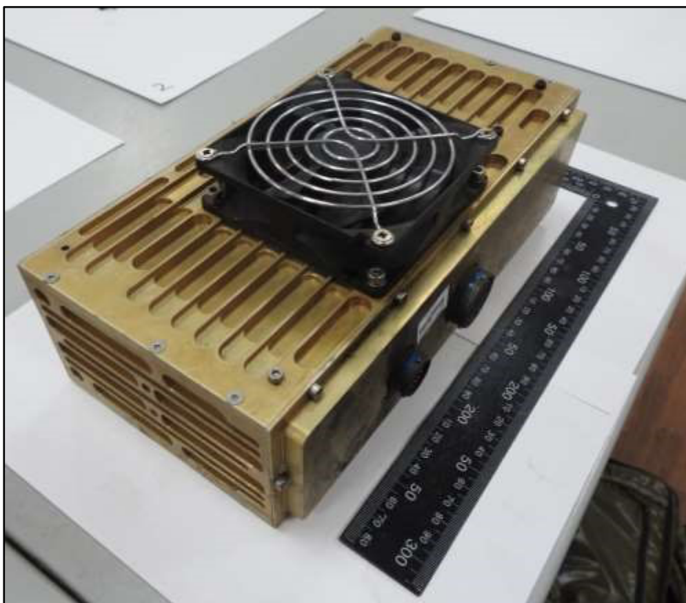
Figure 15. Power Distribution Unit (PDU).
