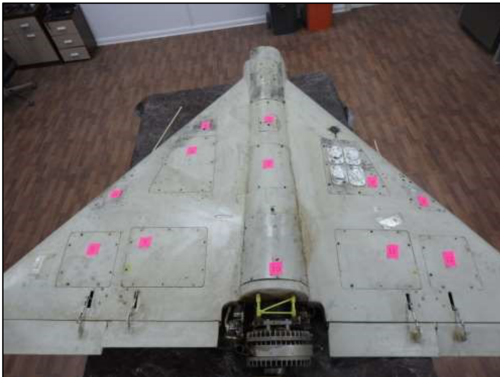
Figure 3. IRN-05 main fuselage with panels labelled.
