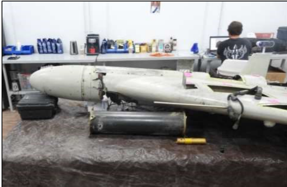
Figure 2. IRN-05 (Shahed-131) rebuilt showing warhead.
