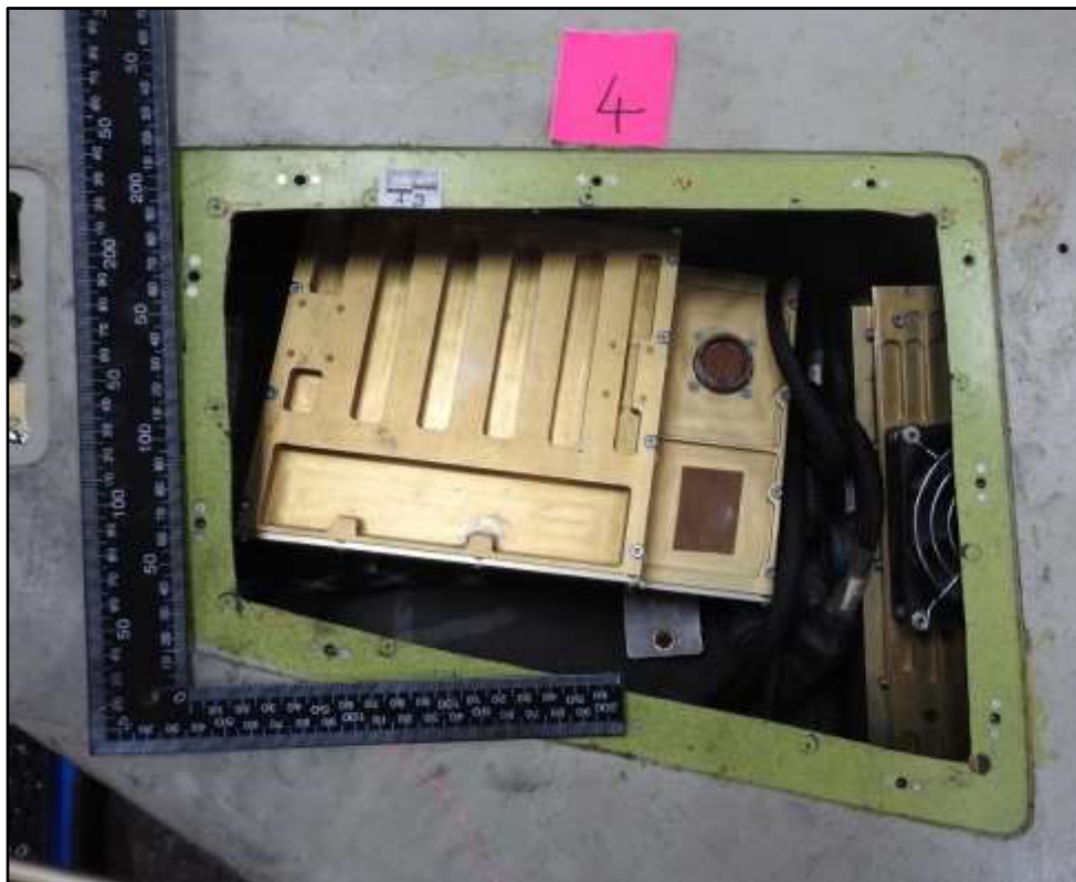
Figure 12 Panel 4 containing Flight Control Unit (FCU) and Power Distribution Unit (PDU).
