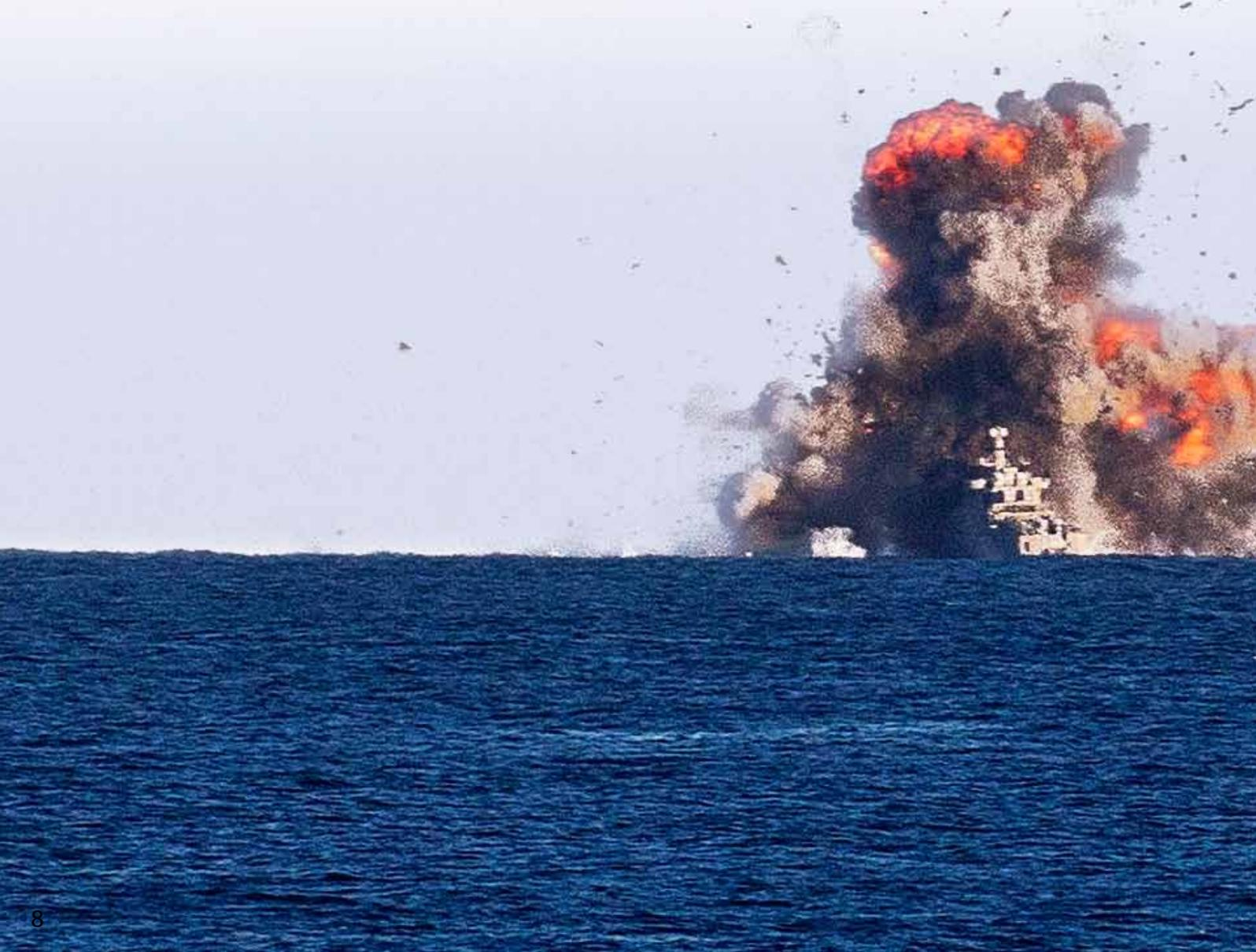
The warhead casing is made of titanium alloy with a steel-grid for fragmentation effect. The picture below shows the warhead effect from a test firing against a Norwegian frigate.
