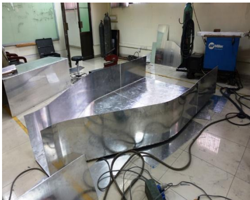
Fig. 5. Contraction Chamber and Setting Chamber
